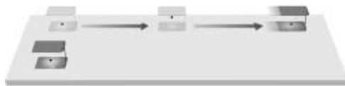
Figure 2.2 A stationary light clock in the foreground while a second light clock slides by at constant speed.
