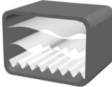
Figure 4.1 Maxwell's theory tells us that the radiation waves in an oven have a whole number of crests and troughs—they fill out complete wave-cycles.
