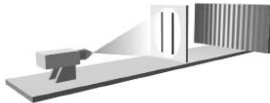
Figure 4.8 If light is a wave, then when both slits are open there will be interference between the portions of the wave emerging from each slit.
